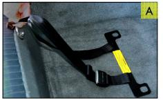
2. Grasp the attachment bracket (Figure B) and (without twisting the webbing) insert it through the vehicle seat bite to the front of the seat (Figures C and D, opposite page).
